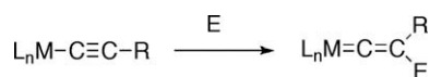
Scheme 2. The formation of a vinylidene from electrophilic addition to a metal acetylide.
